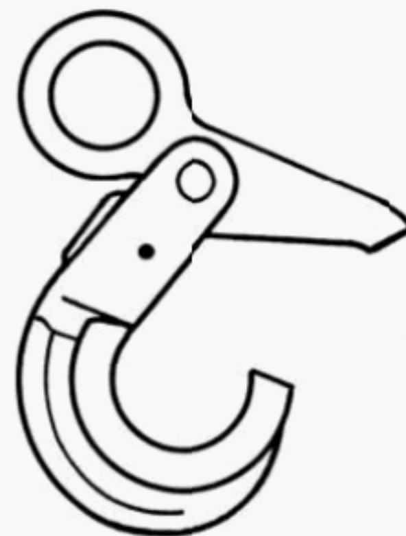
Fig. 10-1.1-6 Self-Locking Eye Hook (Open)
