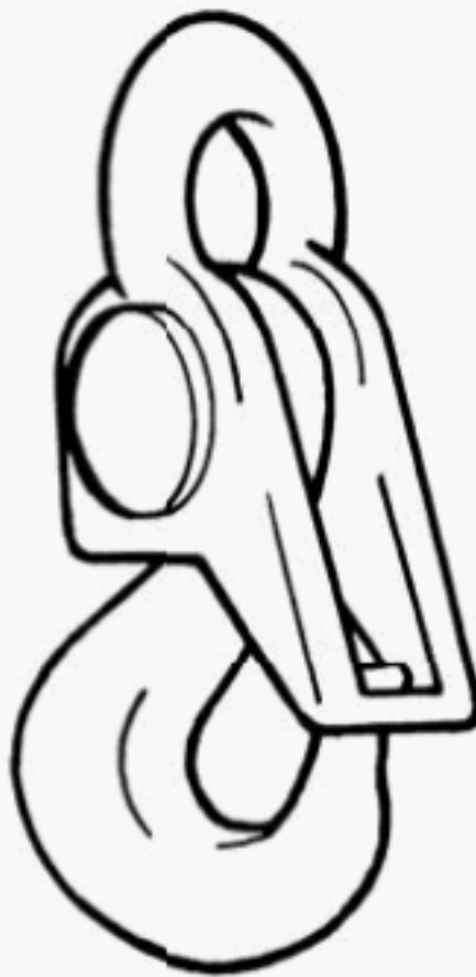
Fig. 10-1.1-8 Self-Closing 8ail (Eye Hook)
