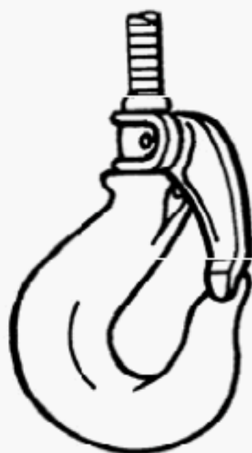
Fig. 10-1.1-9 Self-Closing Gate Latch (Shank Hook)
