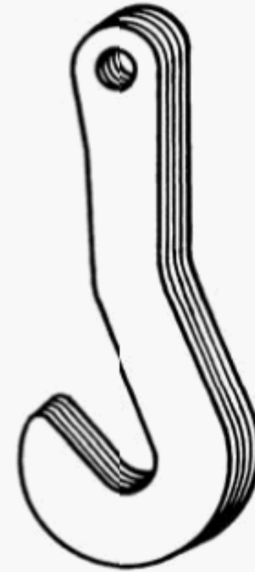
Fig. 10-1.1-16 Laminated Plate Hook
