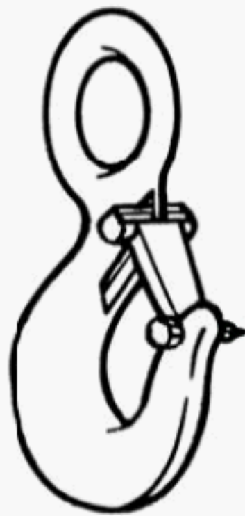
Fig. 10-1.1-14 Self-Closing Tiplock Latch (Eye Hook)
