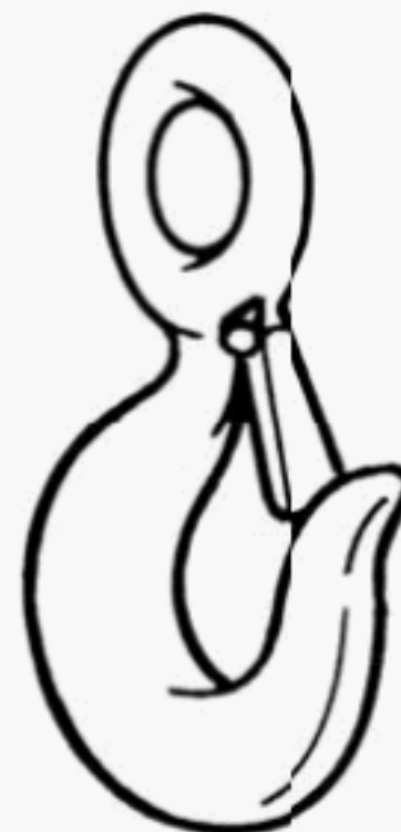
Fig. 10-1.1-12 Self-Closing Flipper Latch (Eye Hook)
