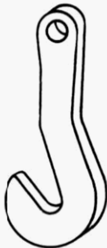
Fig. 10-1.1-15 Single Plate Hook
