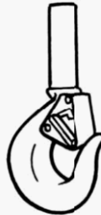
Fig. 10-1.1-10 Self-Closing Flapper Latch (Shank Hook)
